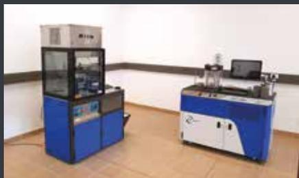
AST for fatigue testing (left) and AMPT for stiffness testing.
