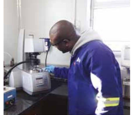
*Lab technician Bonginkosi Xaba uses a Dynamic Shear Rheometer (DSR) to test the rheology of bituminous binders over the in-situ working temperature on the road.*
