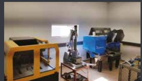
From left: Hamburg Wheel Tracker for rutting testing, coring machine and saw for preparation of samples.
