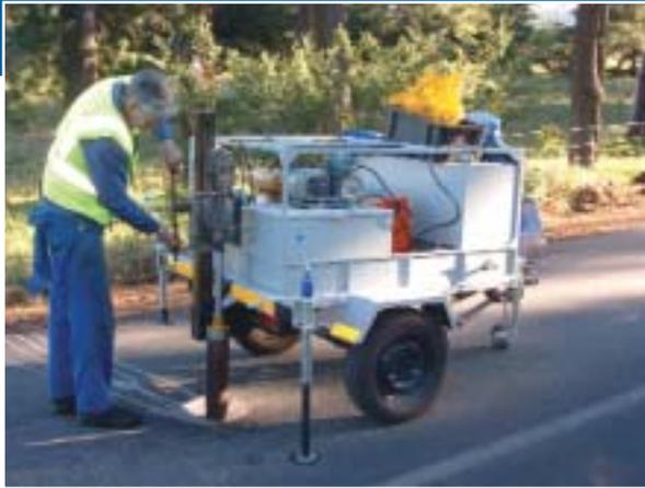
Much Asphalt's Jimmy Henderson cuts cores to check the density of the resurfaced pavement.
