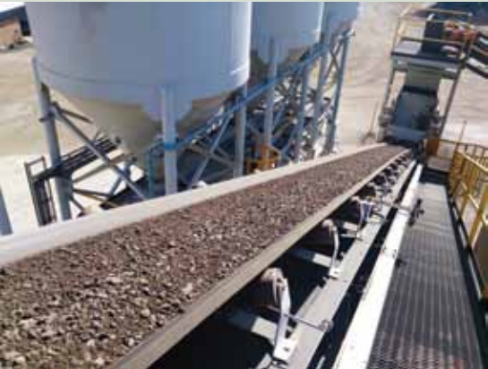
As much RA as the belt will carry continuously going into the plant.
