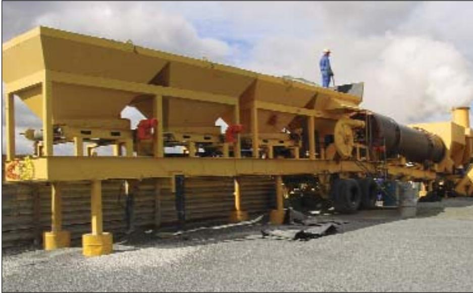
*This Nomad built by CEI in the USA, with a capacity of 120 tonnes per hour, is one of two in Much Asphalt's mobile asphalt plant fleet. A locally manufactured mobile 100 tonne hot storage silo travels with the plant to ensure optimum on-site asphalt capacity.*
