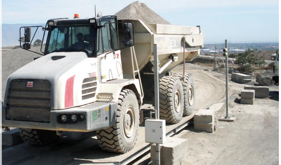
A loaded truck enters Much Asphalt's premises via the unmanned weighbridge.
