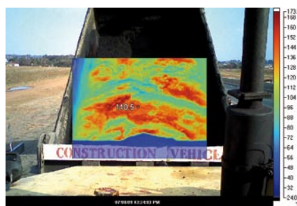
Infrared image of asphalt being tipped into paver
