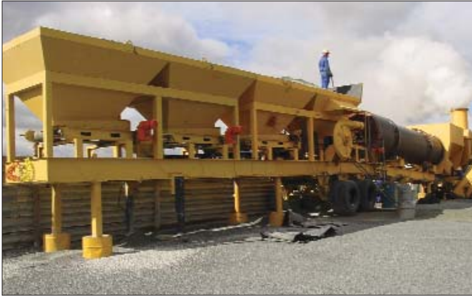
This Nomad built by CEI in the USA, with a capacity of 120 tonnes per hour, is one of two in Much Asphalt's mobile asphalt plant fleet. A locally manufactured mobile 100 tonne hot storage silo travels with the plant to ensure optimum on-site asphalt capacity.
